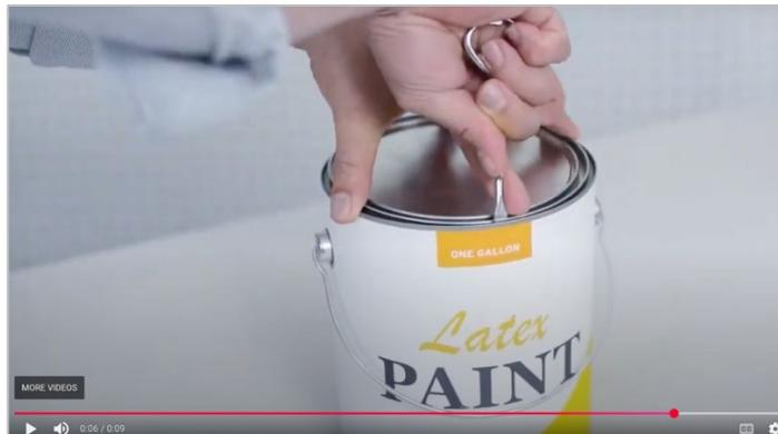
Example of Storage Tip Video Showing Use of a Paint Key or Paint Can Opener Avoid Damaging Can
